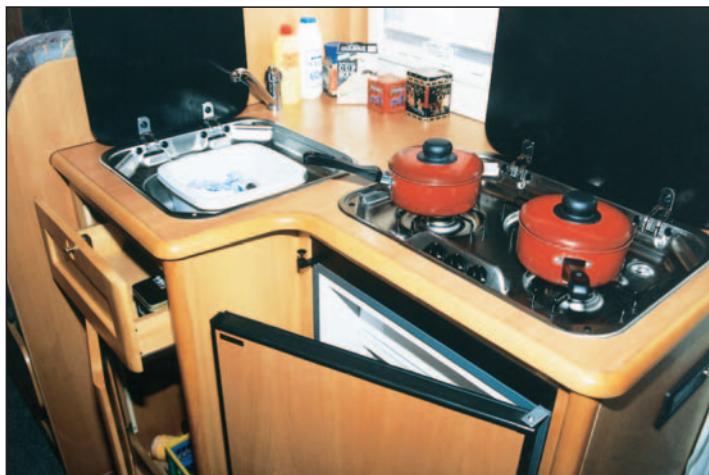
L-shaped kitchen consists of three-burner hob, sink and large compressor fridge. High-level oven is out of picture.
