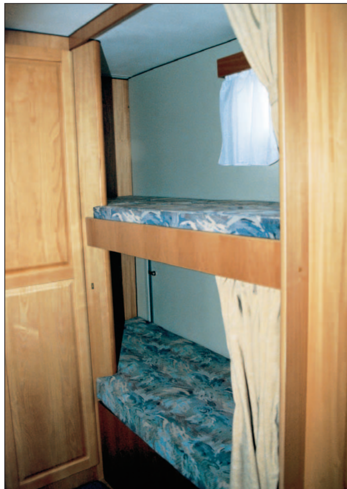
Rear bunks were comfortable. Top bunk is fixed but lower hinges upwards to create large stowage with exterior access.
