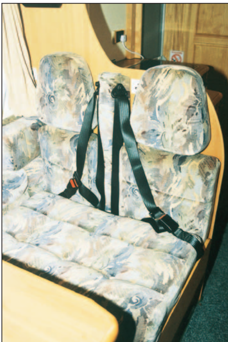
Only two rear seatbelts, despite sleeping accommodation for seven, and rear seat lacks steel support.
